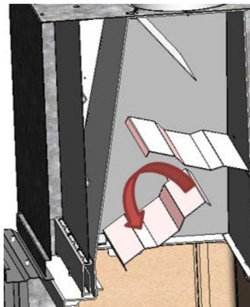
Figure No.31 - Dismantling the lower Itaca 80 eco deflector
